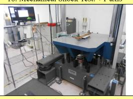
12. Mechanical Shock Test: +Z axis
